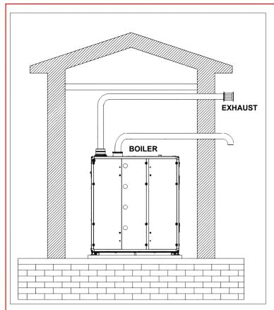
Fig. 33 <u>Sealed Combustion</u> Located on Same Side with Exhaust (horizontal)
