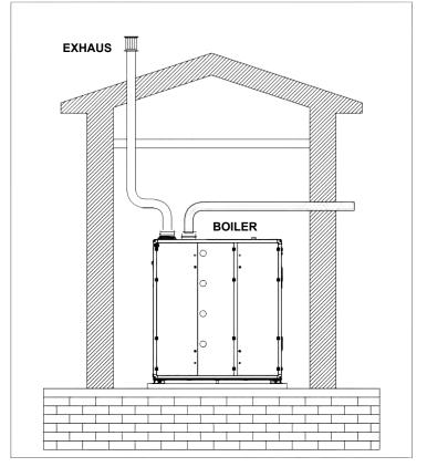
Fig. 34 Sealed Combustion Located on Side Wall
