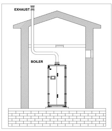
Fig. 31 AII Combustion Air from Outdoors through Single Combustion Air Opening
