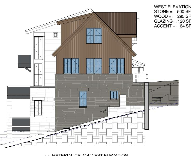
4 MATERIAL CALC 4 WEST ELEVATION 1/8" = 1'-0"
