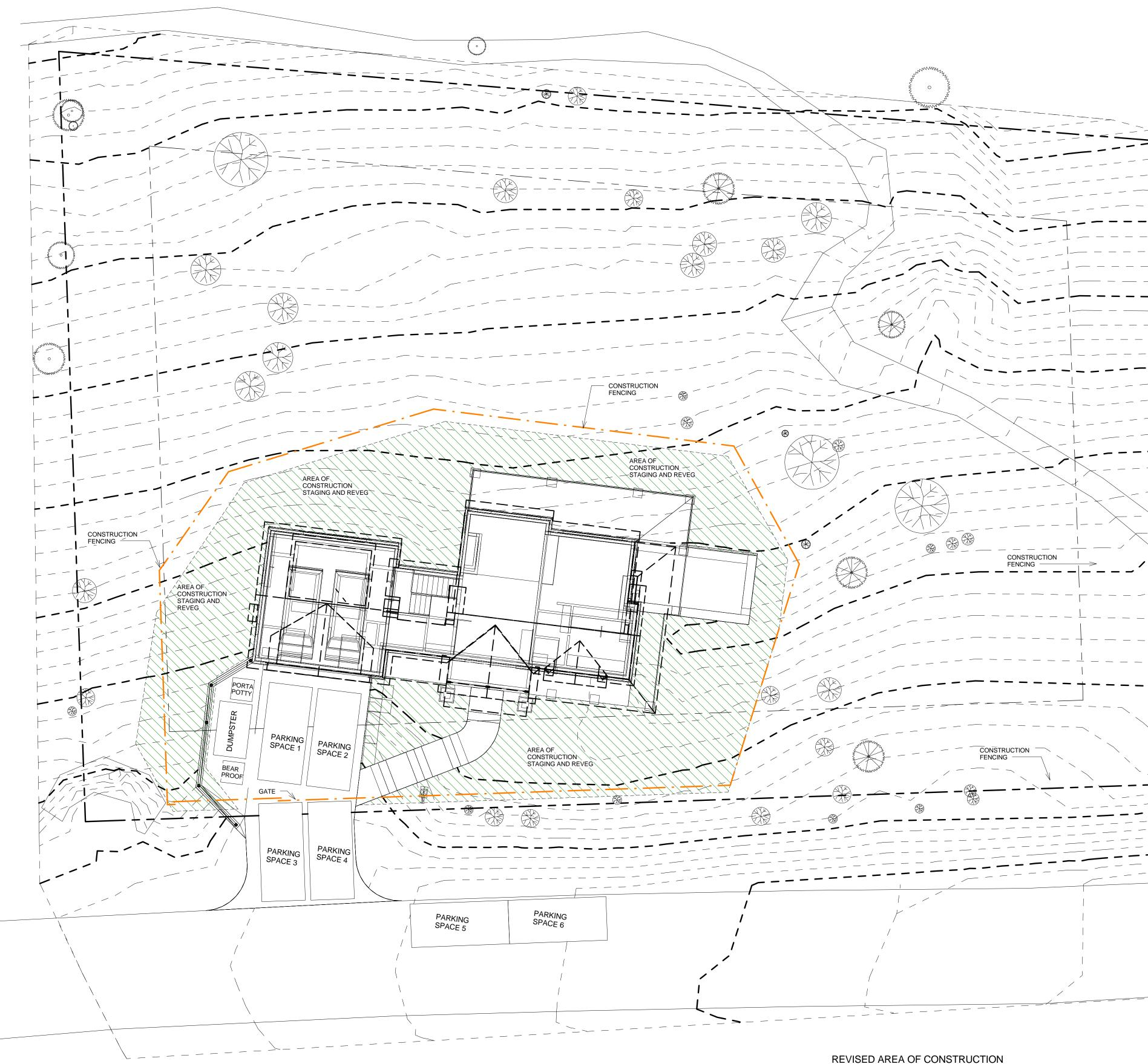
$1 \frac{A101-CONSTRUCTION STAGING PLAN}{3/32" = 1'-0"}$
