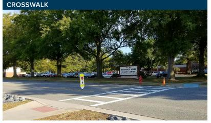
Crosswalk improvements can include pavement striping, curb ramps, striping, signage, and flashing beacons, among others.
