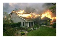
A spark from a forest fire has a high probability of igniting a cedar shake roof, a much greater hazard to an existing home or building than the adjacent forest fire. As noted previously combining a non-flammable roof and defensible space is the optimal means to protect a home in the event of a forest fire.
