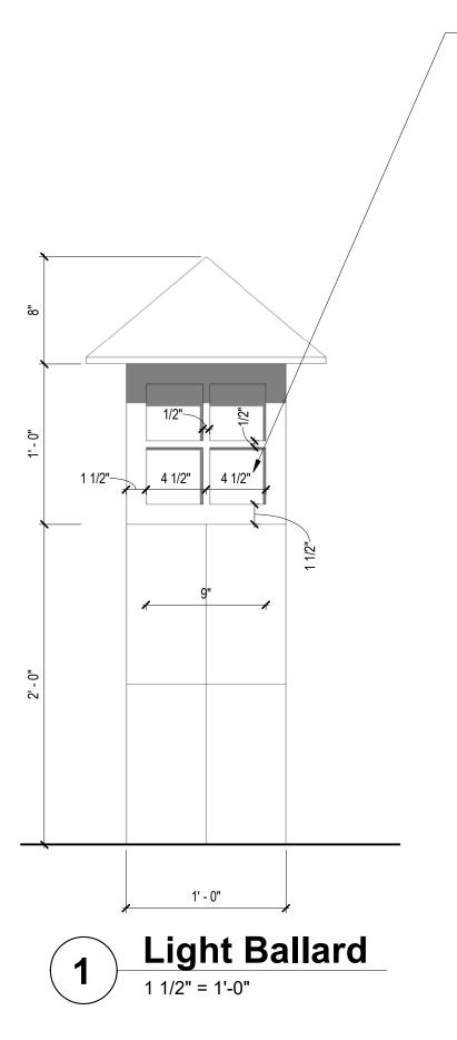
NOTE: OPAQUE GLASS PANELS TO BE PLACED IN THE DESIGN WITH FULL 40W CUT & DOWNLIT LED LIGHT LOCATED INSIDE THE BOLLARD. THESE LIGHTING BOLLARDS ARE FOR SAFETY AT THE STEEP DRIVE, AND ARE MINIATURE MATCHES OF THE EXISTING LARGE ADDRESS MONUMENT CURRENTLY IN PLACE AND EXISTING.
